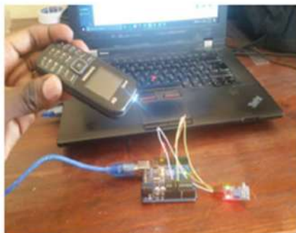
Figures 29 and 30: Showing the Photosensitive Sensor Module Connection – Day Ligh ON, Photosensitive Sensor Module Connection – Day Light OFF respectively.
