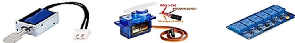
Figures 16, 17 and 18: The 12V Solenoid Lock, Servo Motor SG90 & 6 Channel DC 5V Relay Module respectively.
