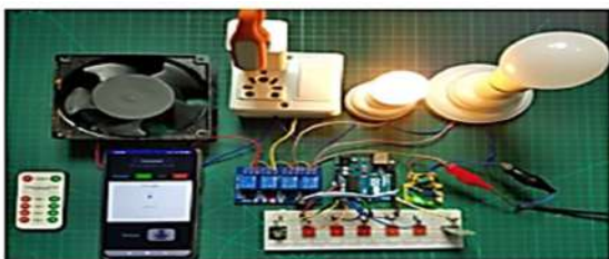
Figures 35 and 36: Arduino Uno integrated with Android (Control), Relays, Loads (Switches), Fans, Bluetooth HC-06, MQ-2 and Photosensitive Sensor & Arduino Uno M-2560 Starter Kit Price (Jumia, 2024)
